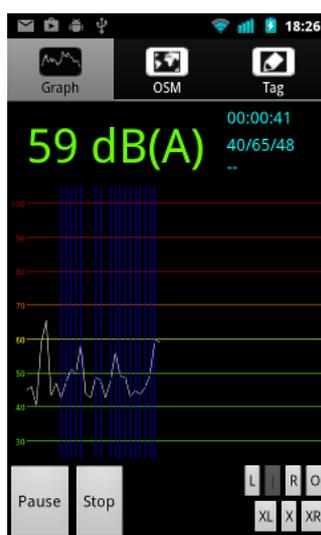
Figure 2. Measuring screen of MobileNoise noise meter application for smart phones. On the right side are buttons for setting position in street network: Upper row sets position on the street (left, center, right, out of street), lower row sets behaviour on crossings (turning left, going straight, turning right). On the left side are buttons controlling measurement itself. Blue lines indicates assigned metadata information.
