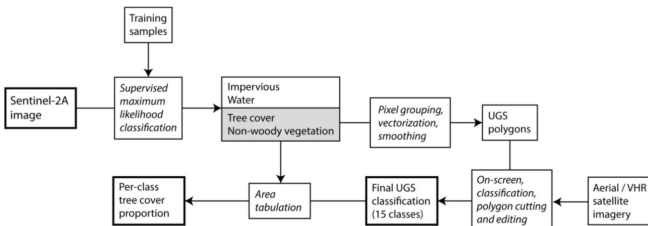
Figure 1. Scheme of the proposed methodology
